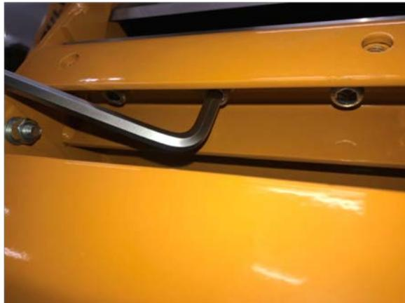
5. Put the anvil back to the chipper and screw on (make sure to keep anvil bolts loose as you need to adjust it later).
