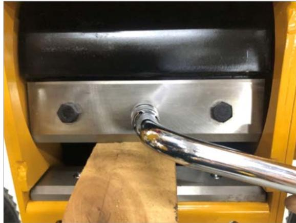
4. Remove the blade anvil (Figure 15). Give a really good clean of chipper blades and anvil and make sure there is no dirt.
